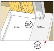
N. **Apply sealant at nosing ends** continuing from the front of the sill pan around the exterior surface of the wall where the sill nosing will end.
